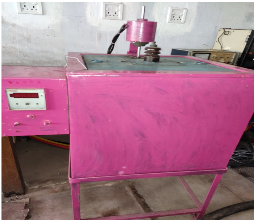
Name of Instrument : Water Bath Uses : Testing Cables as per IS 694 & IS 7098
