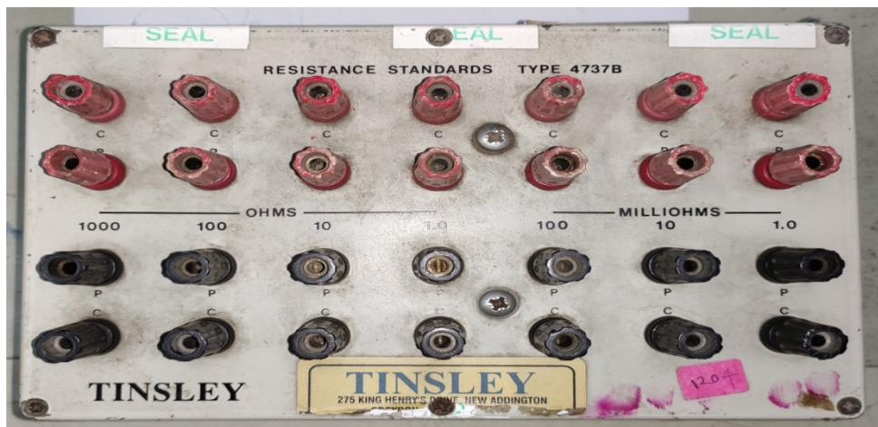
Standard Resistance Box Calibration of Micro Ohm meter / Earth Tester
