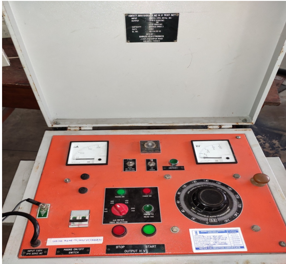
Name of Instrument : AC High Voltage Test Set Uses : Testing Cables as per IS 694 & IS 7098 & 16102 (Pt-1)
