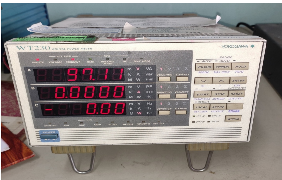
Name of Instrument : Digital Power Meter 3 Phase Uses : Calibration of Power , Harmonics , Power Factor etc
