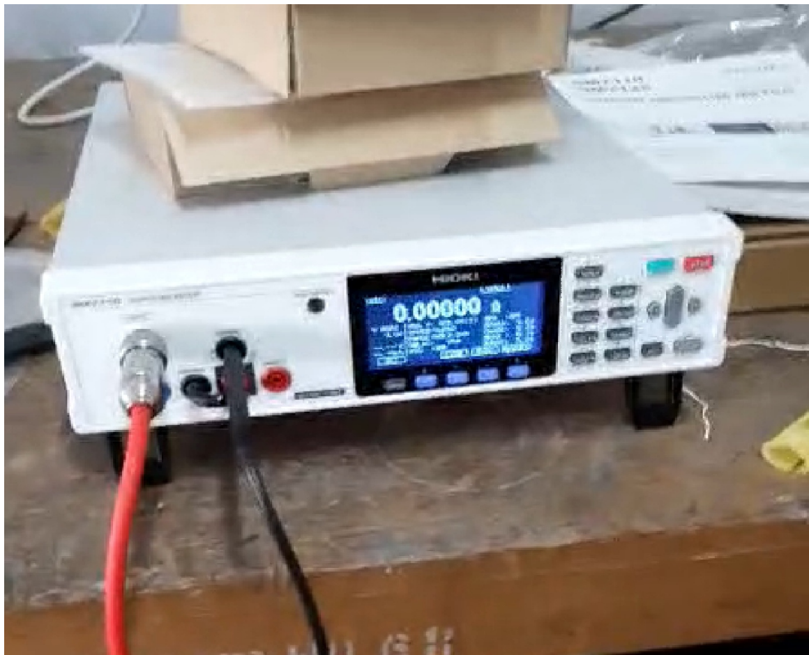
Name of Instrument :Digital Megohm Meter Uses: Testing of PVC and XLPE Cables as per IS: 694 & IS:1544(PT-1),IS:7098(Pt-1)
