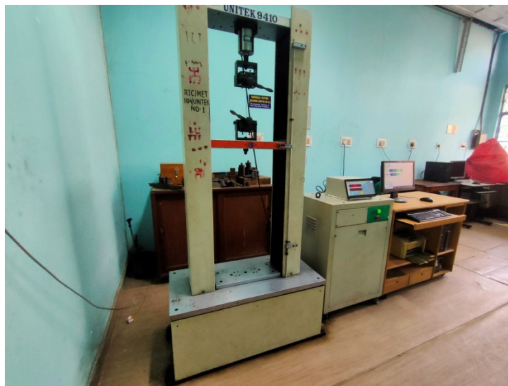
Universal Testing Machine, Cap. 10 KN
