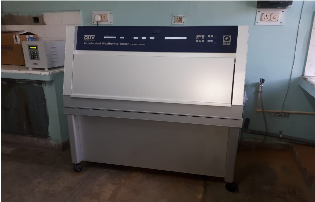
QUV- Accelerated Weatherometer Uses: Durability test of Paint
