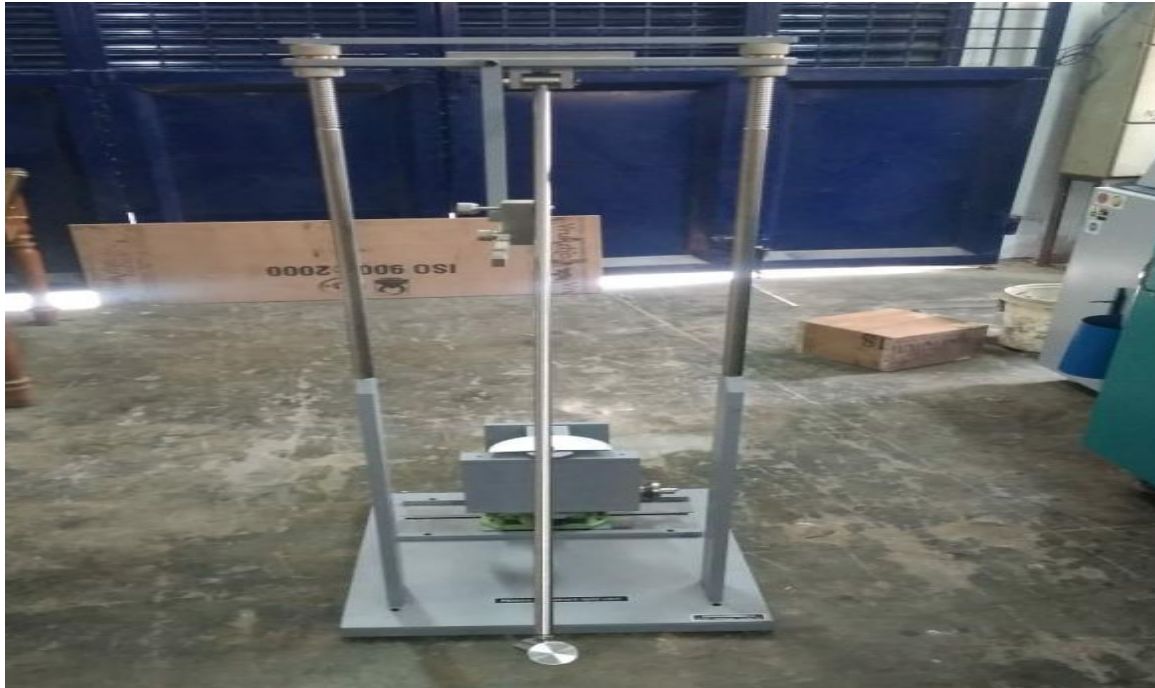
Name of Instrument : Pendulum Impact test apparatus Uses : Testing of LED Luminaire, Meter box, junction box, LED street light, LED floodlight, Switch Testing.
