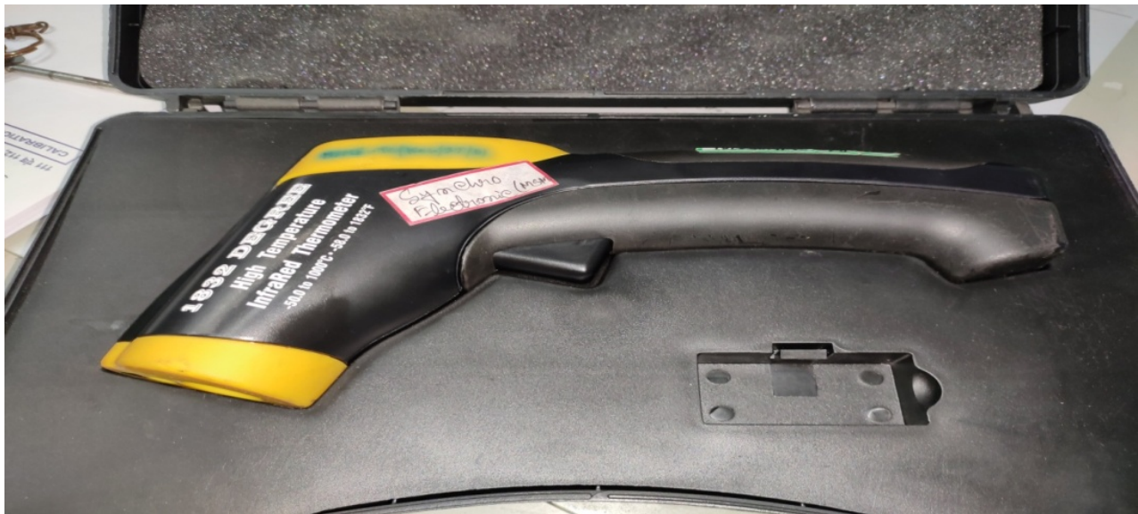
Name of Instrument :Infrared Thermometer Uses : Measurement of Temperature
