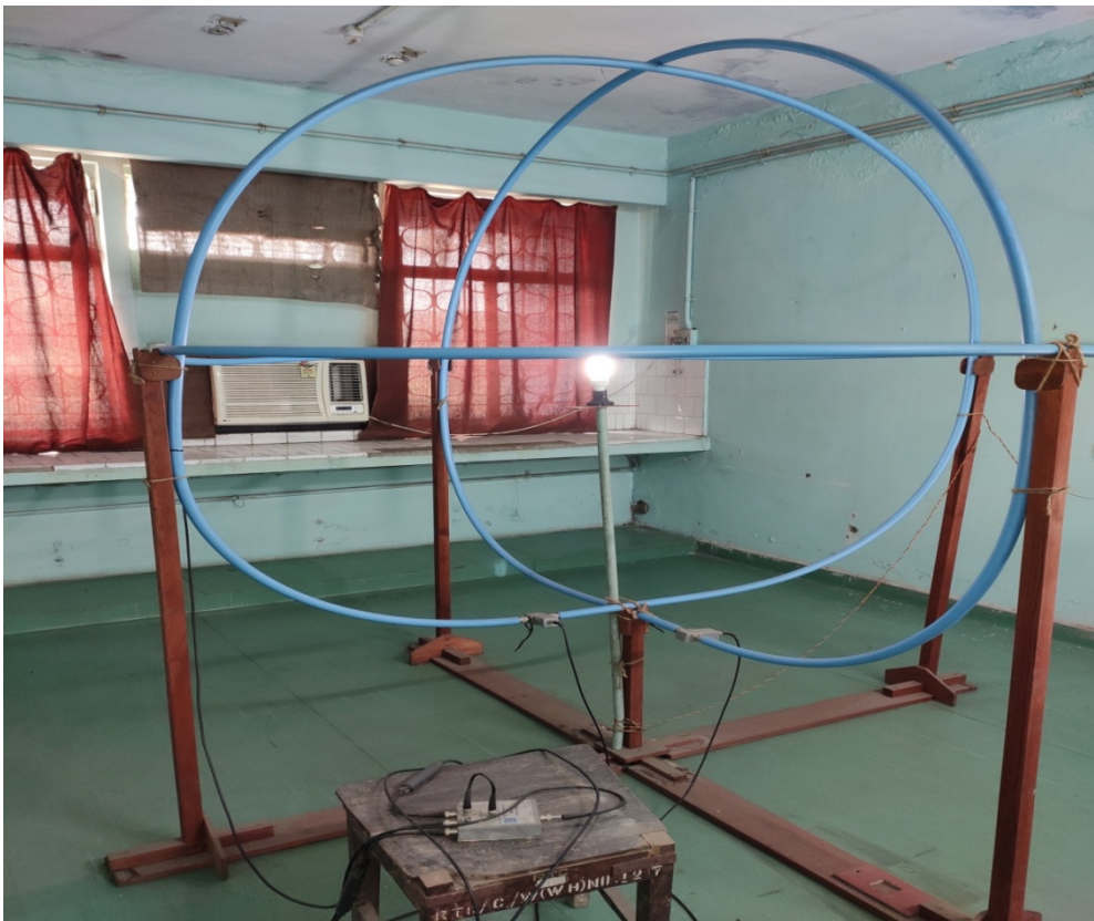
Name of Instrument : Antenna Van Veen Loop Uses : Testing of CFL/LED Lamp
